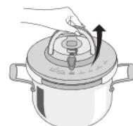
Never force the pressure cooker open, make sure the pressure indicator is down in the normal position.
