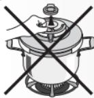
Never remove the Smart Timer® from its housing during cooking.
